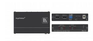
FC-17 is a versatile HDMI 4K@60Hz (4:4:4/4:2:0) converter tool. FC-17 can convert from 4:4:4 to 4:2:0 color sampling and offers EDID management via a user-friendly Windows application. It also enables inter-operability between HDCP 2.2 and HDCP 1.4 systems. FC-17 acts as an HDMI extender that equalizes and reclocks TMDS data before re-transmitting, thus increasing the HDMI cable range from the output
